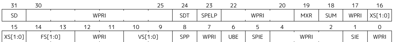
Figure 17. Supervisor-mode status (sstatus) register when SXLEN=32.
